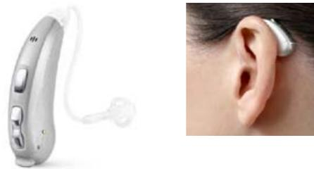
Behind-the-Ear hearing instruments are inconspicuous and comfortable as they do what the name says: they sit behind the ear. BTE hearing instruments are available in two variants: with a tube that delivers the sound from the hearing instrument into the ear, or with an external receiver that sits directly in the ear canal. BTE hearing instruments are available in different performance levels and in many individual colors and designs.
