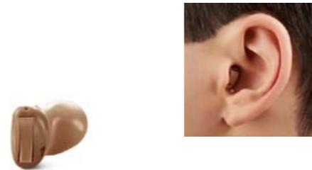
In-the-Ear hearing instruments are worn directly in the ear. They are custom-made based on the anatomy of the wearer's ear. They sit either in the bowl of the ear or deep in the ear canal.
